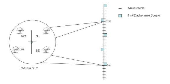
Figure 5. Plot arrangement used for vegetation surveys. The transect line is 25-m long, marked at 1-m intervals for line-intercept sampling. Herbaceous ground cover in a  $1-m^2$  square quadrat was measured at 5-m increments along the transect. At 5 m and 20 m, overstory vegetation was estimated using the point-centered-quarter method.
