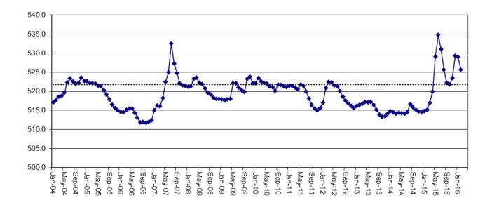
Figure 1. Mean monthly water level elevations in feet above mean sea level (MSL) recorded for Lewisville Reservoir, Texas from January 2004-April 2016. Dashed line indicates conservation pool (522 feet above MSL). Data were obtained from the USGS.
