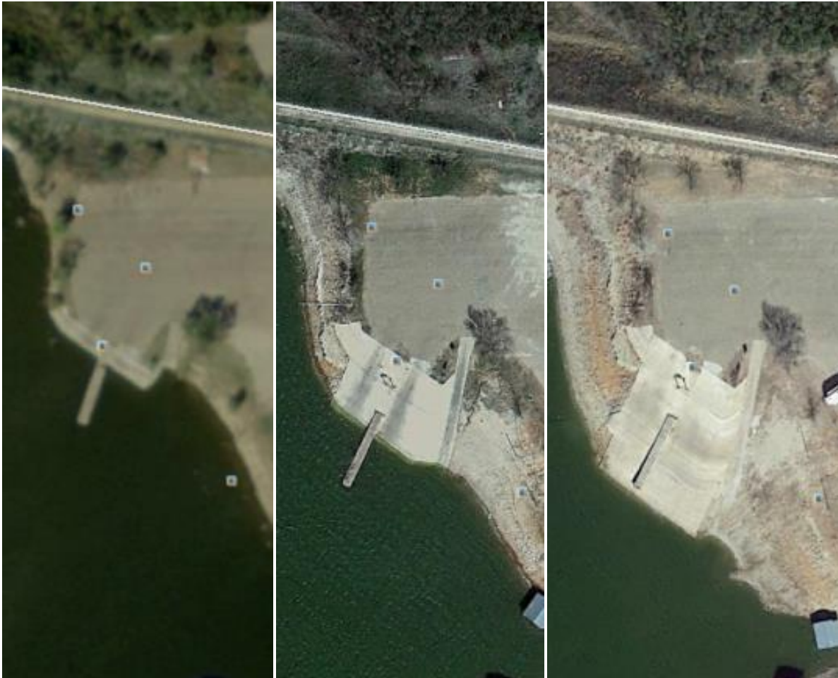
Google Earth satellite images of the public boat ramp on Sweetwater Reservoir, Texas, imagery dates ranged from 10/30/2008, 2,113.0 feet above mean sea level (left) to 1/25/2014, 2,092.7 feet above mean sea level (right) (accessed 11/14/2014). Conservation pool at Sweetwater Reservoir is 2,116 feet above mean sea level.
