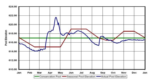
Figure 2. Example of the seasonal pool elevation management plan for Texoma Reservoir 2008.
